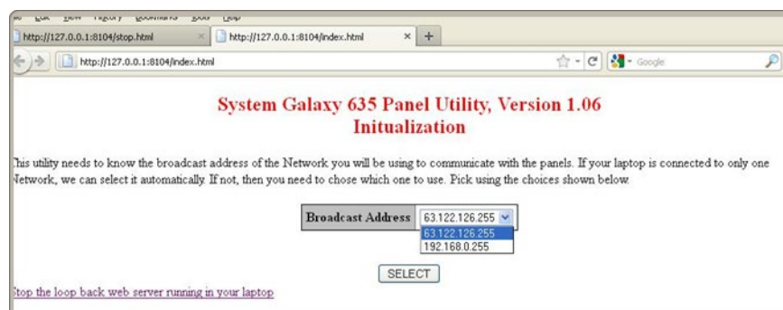
Figure 43 – Example of 635 Web Config Tool Screen
